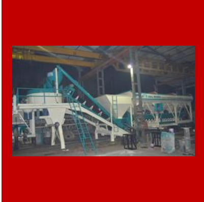
Concrete Batch Mix Plant
